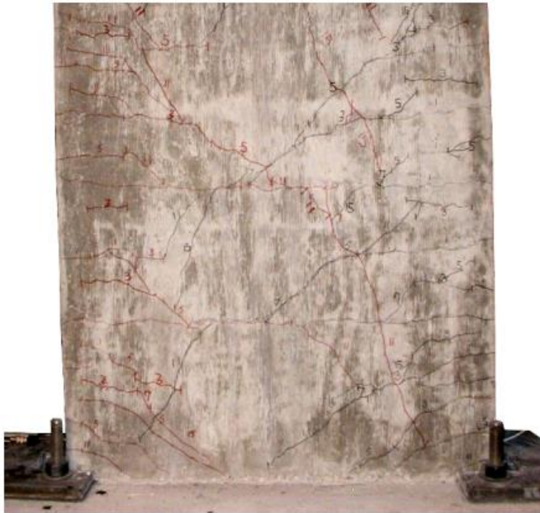
a) Reinforced concrete wall
