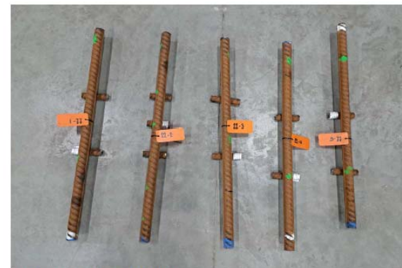
Samples 22-1, 22-2, 22-3, 22-4, 22-5 after fatigue
