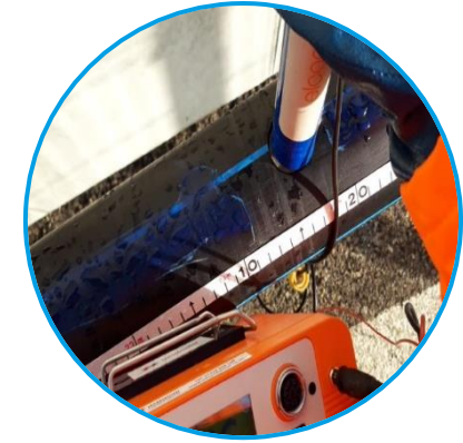
Half cell potential measurement
