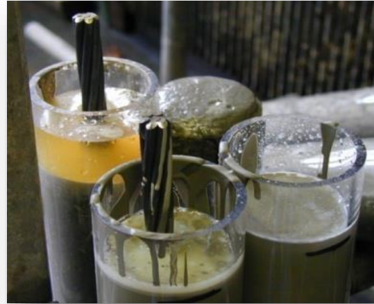
VSL tests of grout mix
