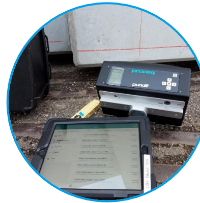
Ultrasonic Pulsed Echo
